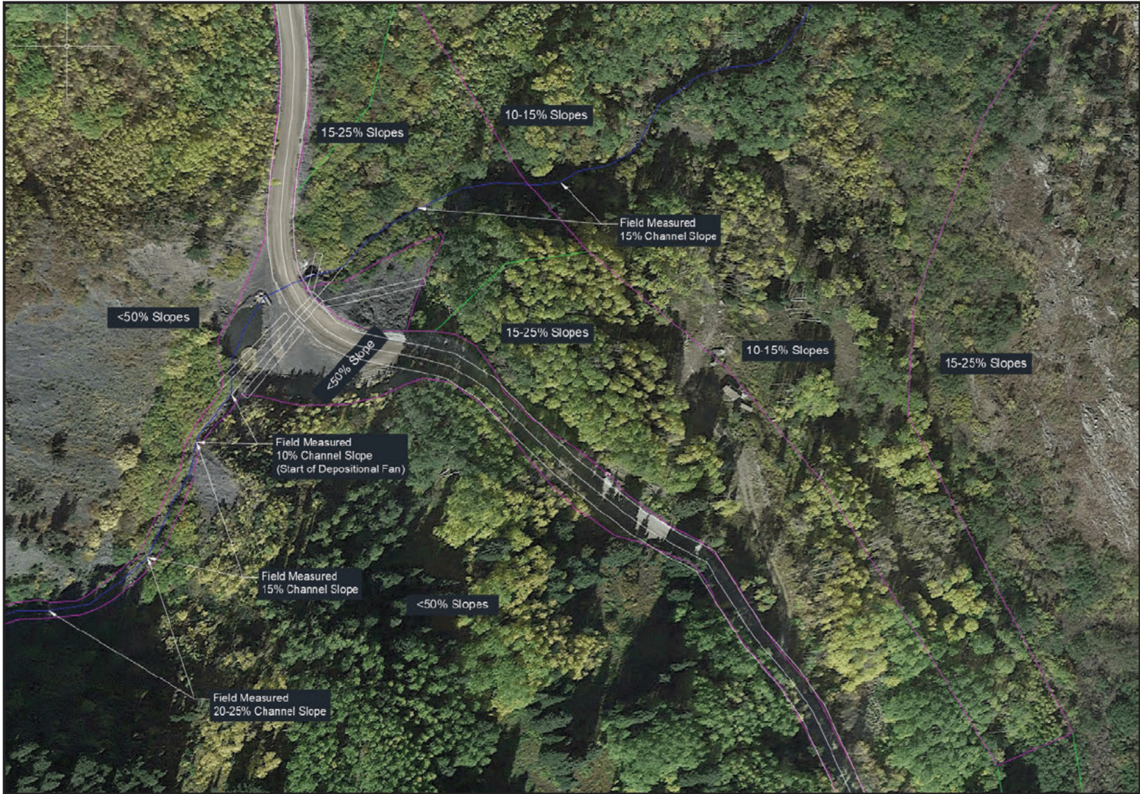
Figure 3. Existing channel slopes over a GoogleEarth image captured October 2019. North to top of image.
